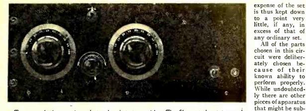
Two controls that require only two hands to tune with. The filament rheostat may be set and left there, and while the regeneration requires an occasional touch when tuning on widely separated wavelengths, it is not troublesome. The filament switch on the right permits one to turn off the set while lashing the phones or loud speaker to the table when strong signals are to be received.
